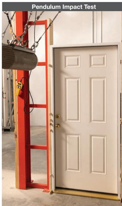
Pendulum Impact Test
